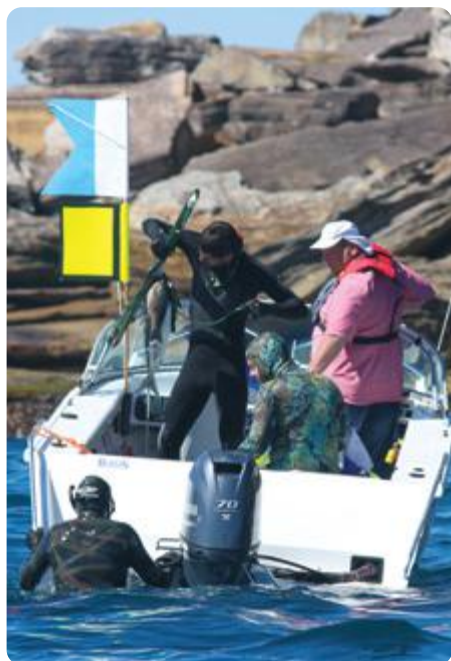
The blue and white 'Alpha' flag can be attached to a vessel.
